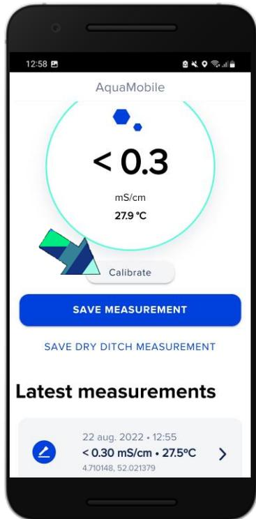
Select "Calibrate" to start EC calibration. The EC calibration requires calibration fluid of 0.01 M KCl, 1.413 mS/cm.
